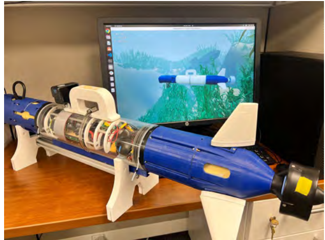
Fig. 1. A CougUV robot is tested in the lab prior to field trials with a HIL setup with the HoloOcean simulator. Where simulated sensor data is sent to the CougUV and processed onboard. Control surfaces are actuated and commands are sent back to the simulator, where the vehicle's motion is calculated.
