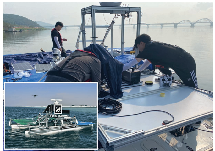
Figure 3. Testbed USV used for dataset acquisition in the SPC-presented paper, modified and operated by the Mobile Robotics & Intelligence (MORIN) Lab at the Korea Advanced Institute of Science and Technology (KAIST).
