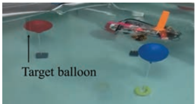
Figure 5. An example of balloon recognition using Hough transform. The recognition result was almost perfect but not robust against other objects.
