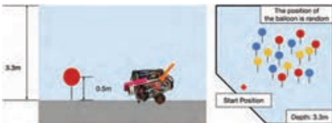
Figure 2. Overview of water tank setup.
