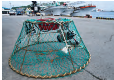
Figure 5. Deep-sea camera system for red crabs.
