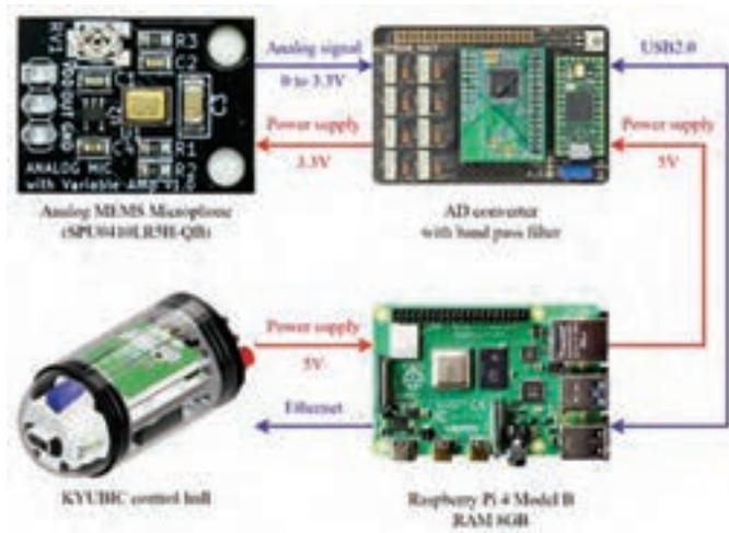
Fig. 5 Device connection.
