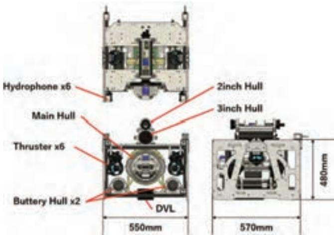
Fig. 4 General arrangement of AUV KYUBIC.
