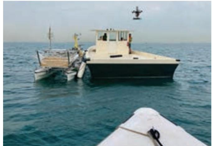
*Drone picking up the object after USV has autonomously docked to the target vessel.*
