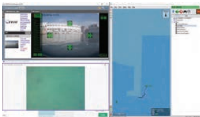
The view on the operator screen displaying an above-water camera stream, underwater-camera stream, and Neptus GUI with a position of the robot in the surrounding area.
