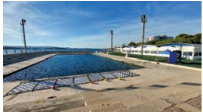
“Ocean pool” that served as testing grounds—the used fish cage net with hand placed patches can be seen.
