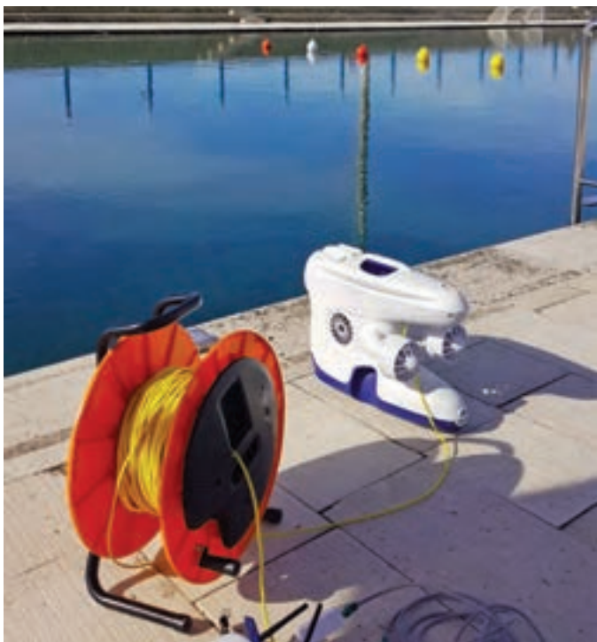
The used underwater ROV behaved well under autonomous control, supported by an underwater localization system to close the control loop.
