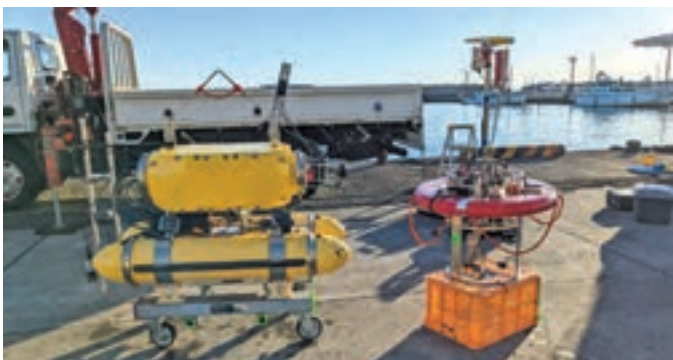
Figure 6. The crane truck with the AUV and the buoy.
