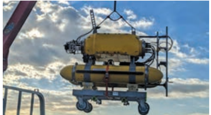
Figure 7. The scene of lifting up the AUV by the crane truck.
