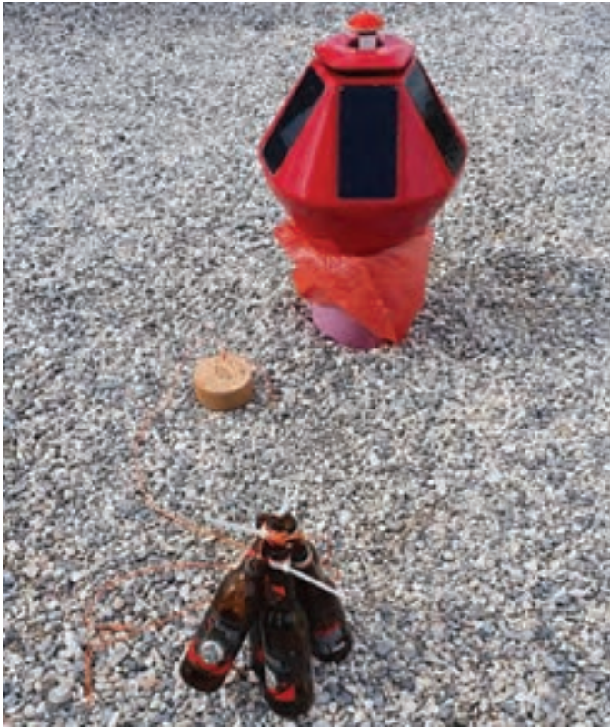
Smart Buoy prepared for deployment along with marine litter attached to a floater, which served as the mission target.
