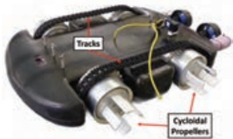
Fig. 1: Cyclo-propeller Unmanned Underwater Vehicle (Cyclo-UUV).
