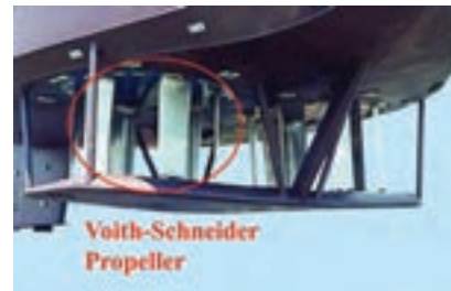
Fig. 2: Voith Schneider Propellers mounted on a tugboat.
