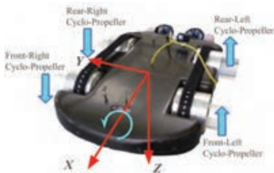
Fig. 12: Differential thrust vectoring being used to generate a positive rolling moment.
