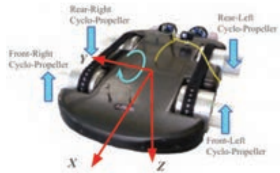
Fig. 13: Differential thrust vectoring being used to generate a positive pitching moment.
