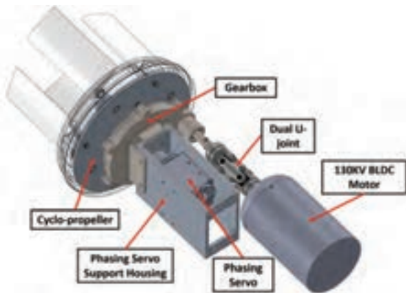
Fig. 9: Cyclo-propeller drivetrain render.
