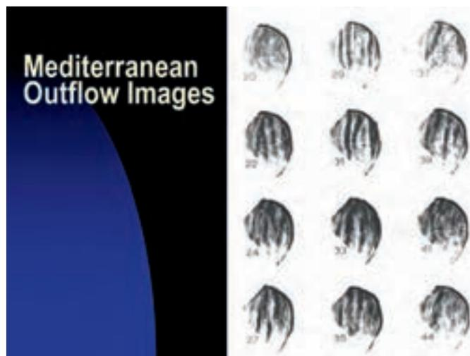
Figure 2. Salt finger shadowgraph images across the interface at 1265 m depth in the Mediterranean outflow. Images are 2 cm in diameter and spaced vertically as shown.
