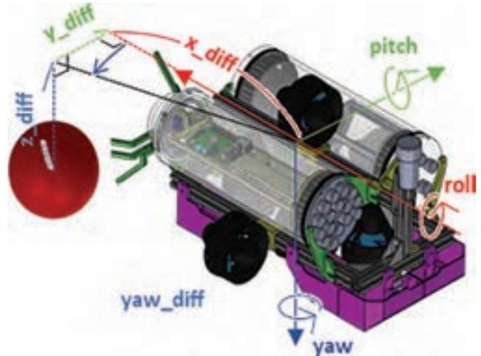
Figure 9. Calculate the position of the balloon considering the attitude of the AUV.
