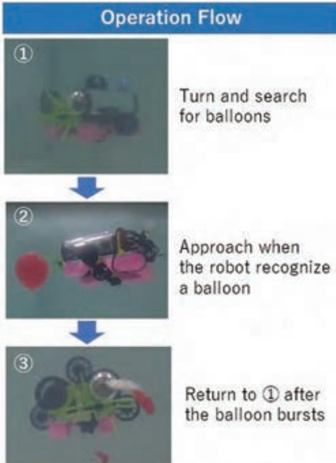
Figure 3. Operation Flow of AUV.
