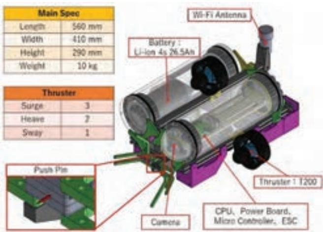
Figure 4. General arrangement of AUV wARIEL.
