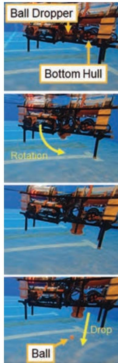
Figure 7. Operating scenes of developed ball dropper.
