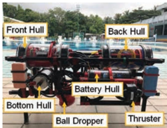
Figure 2. Appearance of AUV Marine Gear.
