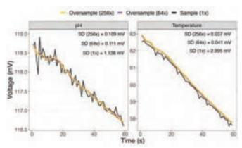
Fig. 2. Oversampling rate comparison between 256x (yellow) and 64x (purple) oversampled data, and 1x (black) sampled data for pH (left) and temperature (right) pins on the new design data logger. Standard deviations (SD) are displayed for each sampling rate. Each time point represents a 10 second sampling period for a total of 10 minutes.
