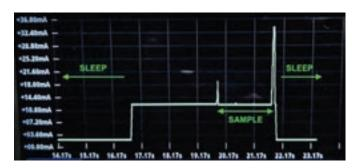
Fig. 6. Current readings from the new data logger design during sleep mode (approx. 2 mA) and while sampling (approx. 12mA).
