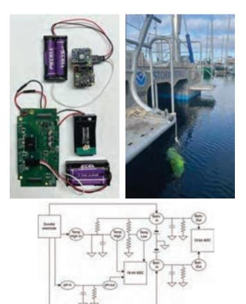
Fig. 1. *Top left*: Side-by-side comparison of old (MadgeTech, bottom) and new (open-source, top) sensor electronics. *Top right*: Packaged sensor systems concurrently deployed in a dive bag for field deployments in Port Angeles Harbor, Washington. *Bottom*: Circuit schematic of the voltage divider circuits joining the pH electrode to the ADC inputs [22].
