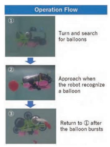
Figure 3. Operation Flow of AUV.
