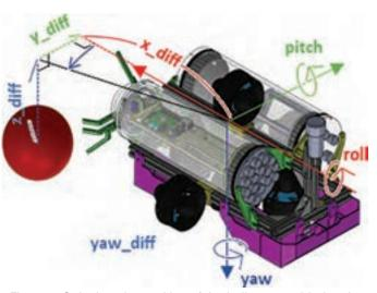
Figure 9. Calculate the position of the balloon considering the attitude of the AUV.
