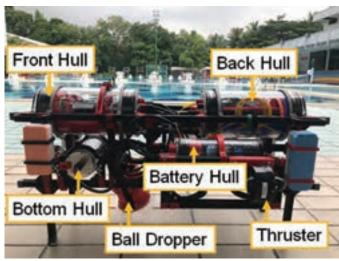
Figure 2. Appearance of AUV Marine Gear.
