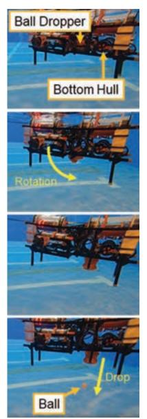
Figure 7. Operating scenes of developed ball dropper.
