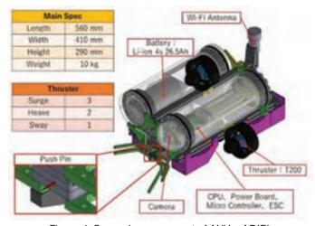
Figure 4. General arrangement of AUV wARIEL.
