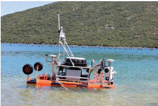
Initial trimming of the ASV Korkyra and manual control tests with Blueeye Pro ROV tied in front of its TMS on Monday, 25th of April.
