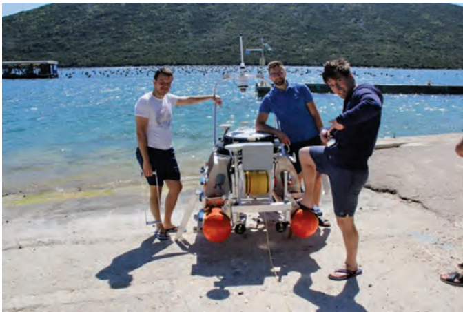
Deployment of the ASV Korkyra is now a 2–4 person job since its weight increased significantly with added subsystems.
