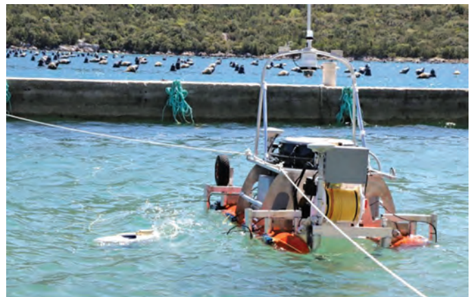
Successful performance tests of TMS-GNSS-UWGPS G2 integration performance tests at sea on Thursday, 28th of April.
