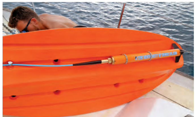
Caution! Engineer at work! Installing a compact magnetometer onto a plastic unsinkable kayak.
