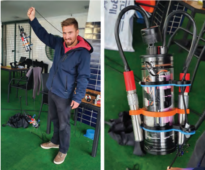
Martin Oreč testing out mooring line attachments for sensor units before deployment.
