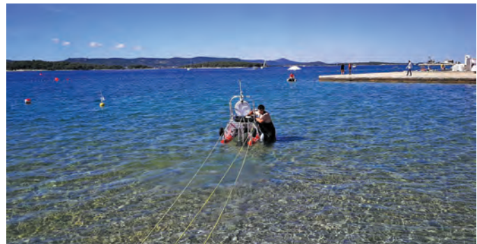
Tying the ASV Korkyra to a pillar at the beach in Biograd na Moru to ensure safety during the thruster power consumption tests.
