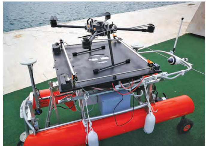
LP performance tests in Biograd na Moru. Manual landing of the UAV and automatic LP open/close actions were a success.
