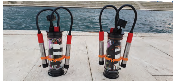
Two underwater sensor units prepared for long-term deployment in the pool at Biograd na Moru.
