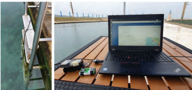
A topside laptop (right) served as a placeholder "buoy unit" in the initial experiments, providing an endpoint for acoustic communication (left).
