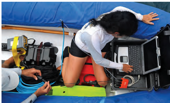
Setting up the magnetometer for towing by the dinghy, with a ruggedized laptop and portable 12 VDC battery box—this is how we found some wrecks!
