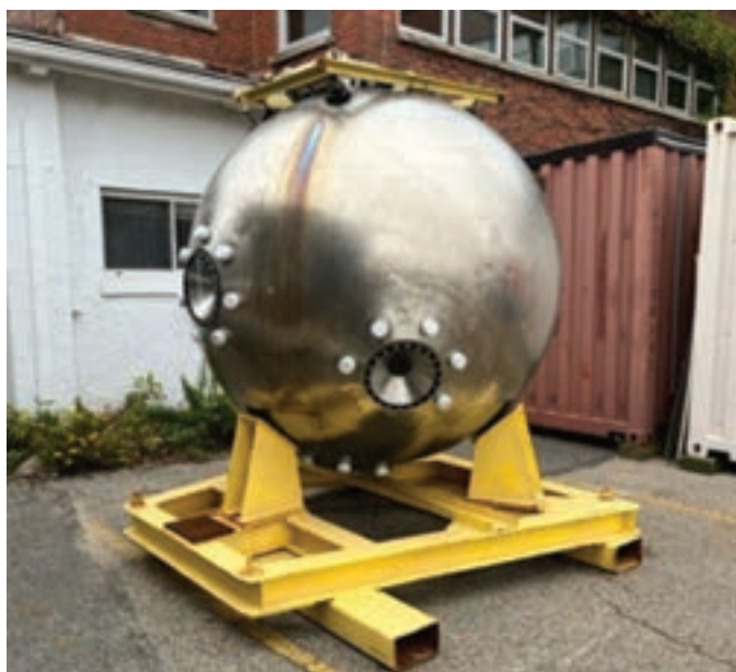
Figure 2. Alvin personnel sphere—Titanium.
