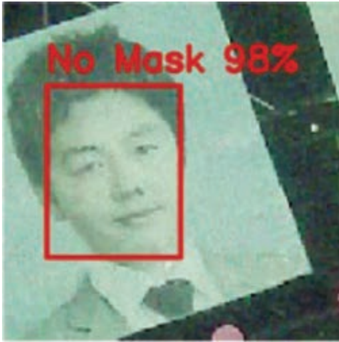
Figure 6. The AI system in ARIEL detecting a non-masked person using a downward looking camera.
