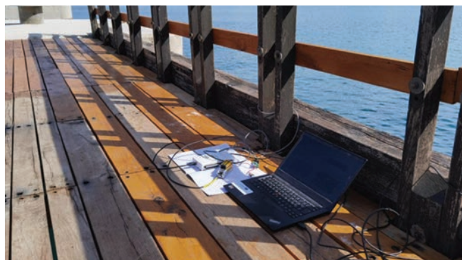
Experiment setup for diver breathing/bubbles detection recorded by a simple hydrophone.
