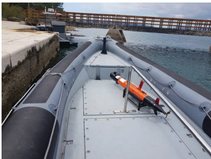
Deployment of LAUV Lupis from the side of a boat.
