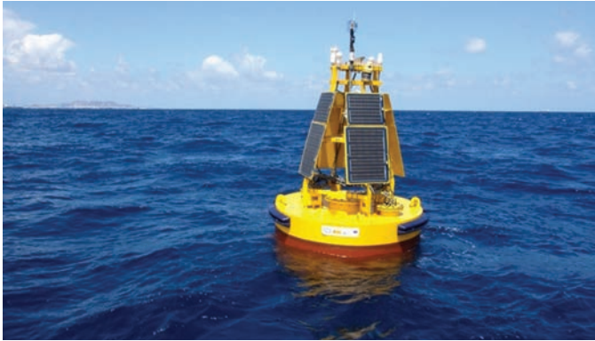
A moored buoy for long-term ocean measurements close to the Canary Islands (© PLOCAN, Spain).
