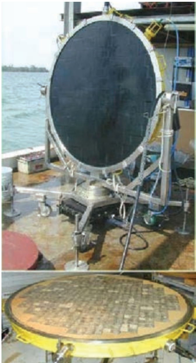
ROMANIS, the 2D ambient noise imaging camera getting ready for deployment (top) and its 508 sensor array exposed (bottom).
