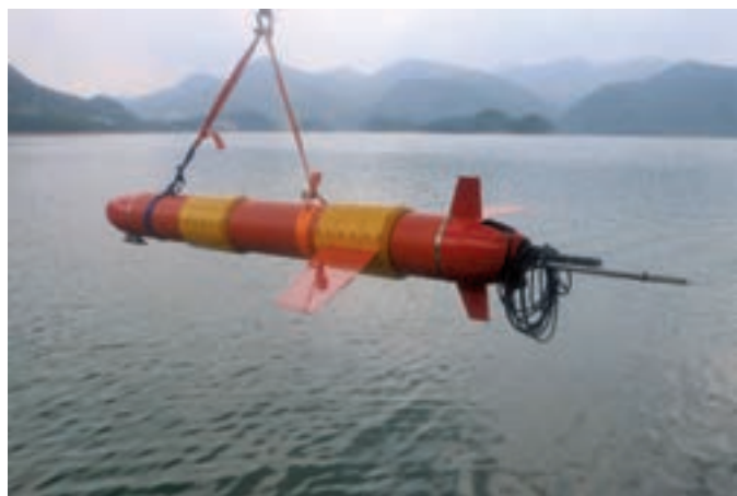
The novel multi-modal underwater vehicle launching from shore.
