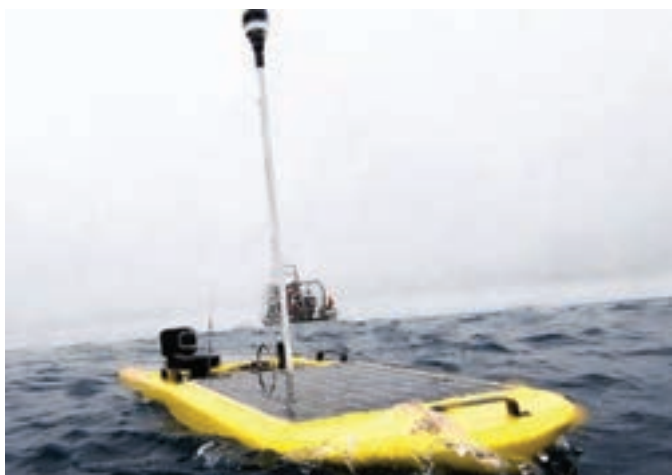
A WaveGlider splashes along, pulling energy from the sun and sea. Solar power converted to electricity is stored in LiPo batteries.
