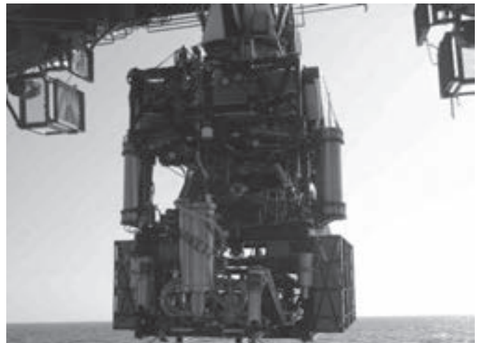
Earthquake and Tsunami Observatory Installation using ROV HyperDolphin.
