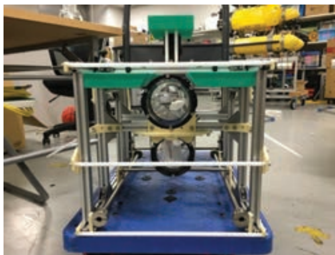
Shafts for adjusting own attitude and buoyancy
