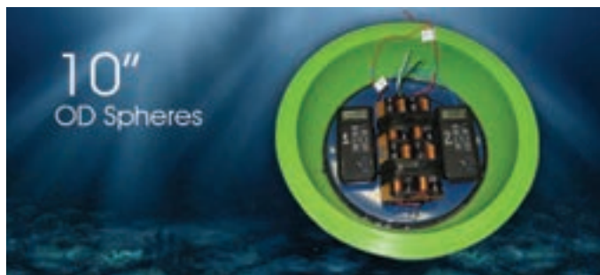
A 10" instrument sphere holds a pair of countdown timers and batteries for a dual burnwire release. (Photo courtesy of Global Ocean Design.)
