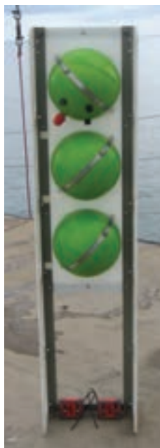
10" Polystyrene spheres in a Nanolander™, on the pier (left), and floating in saltwater. (Photo courtesy of Global Ocean Design.)
