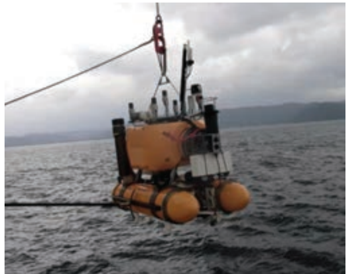
The deployment of the AUV "Tri-TON 2". The AUV navigated based on the station and visually observed the hydrothermal bent field.
