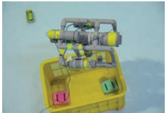
The ROV which was assembled by the participant in the junior section. The robot picks up an empty can on the pool floor.
