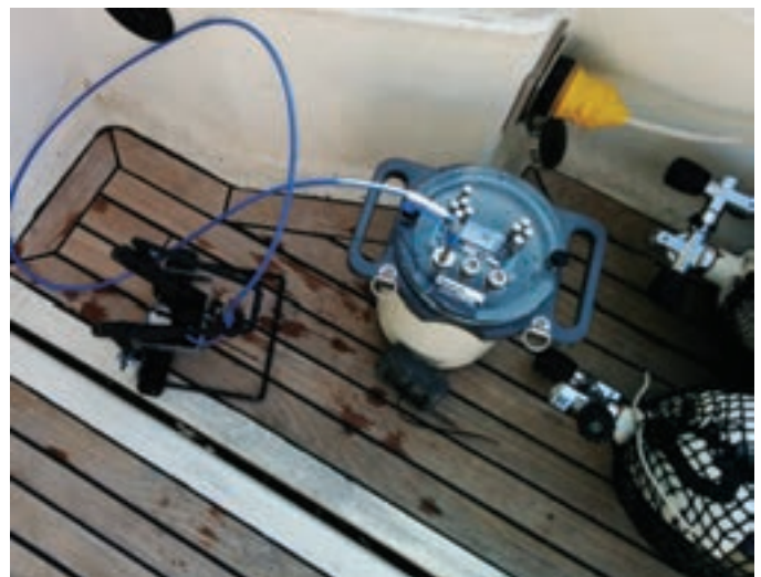
Figure 4: Spectrometer used in collecting seafloor reflectance spectra during a diving operation.
