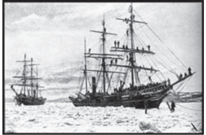
Steam ships similar to 'City of Halifax' in the Newfoundland seal fisheries during the 1860s or 70s. These ships had thick wooden hulls to resist the ice, and were still in use in the 1930s.
