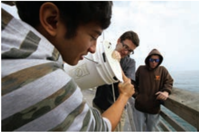
Students pour a fresh seawater sample into a 1 meter glass tube to check turbidity using a variation of the traditional Secchi disk technique.
