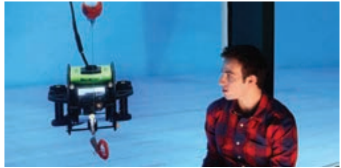
A student gets hands-on experience with a Remotely Operated Vehicle (ROV) in the Marine Institute's Flume Tank. The Flume Tank is the largest in the world and is used to carry out performance evaluations, gear tests and other observations on newly developed or existing fishing gears and other related equipment in simulated underwater and near surface conditions.
