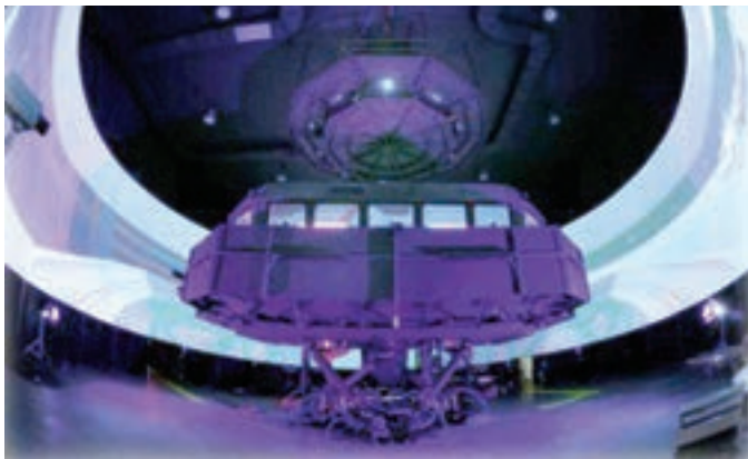
The Marine Institute's Full Mission Ship's Bridge Simulator is used to replicate operations conducted on a ship's navigation bridge. The simulator is mounted on a six degree of freedom (DOF) aviation motion base and is one of two full-motion ship's bridge simulators in the world.
